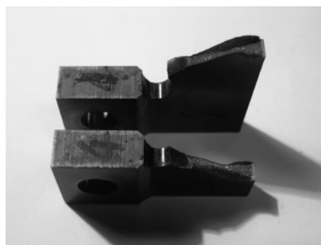
Fig. 11 Picture of a cracked specimen
